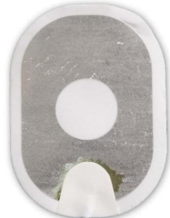
**Figure 3:** Gel almost completely separated from backing.
