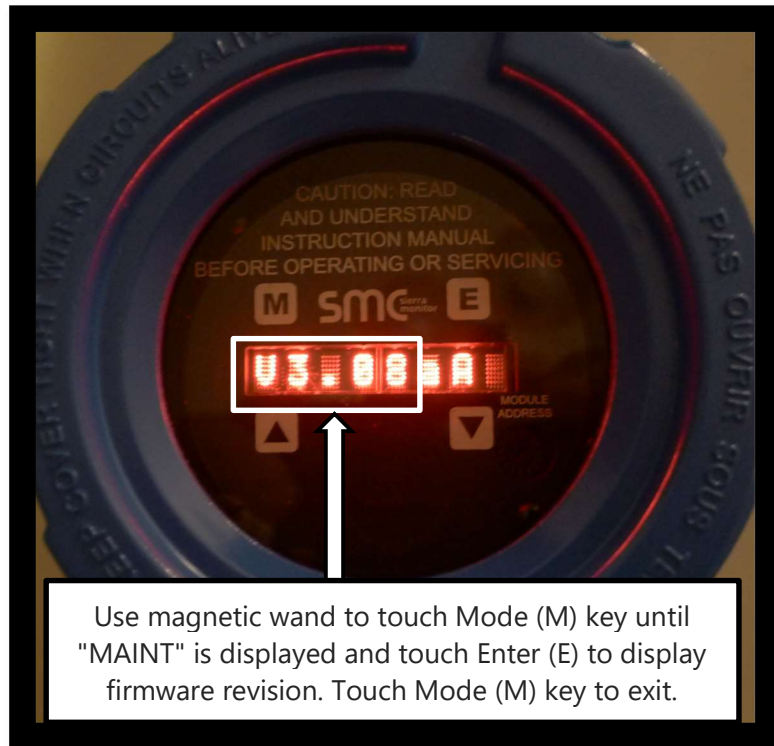
Figure 2 – Firmware Revision Identification for SMC 5100
